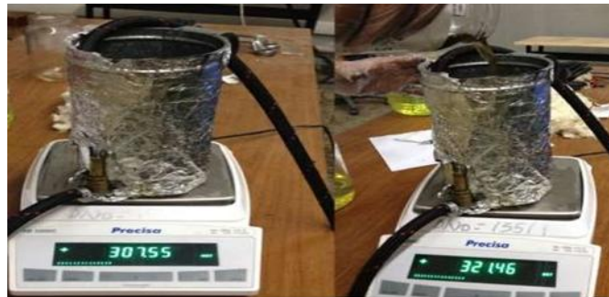
Figure2: Electronic Scale Used in Fuel Consumption
