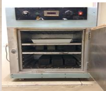
Figure 4: Curing of Cubes
