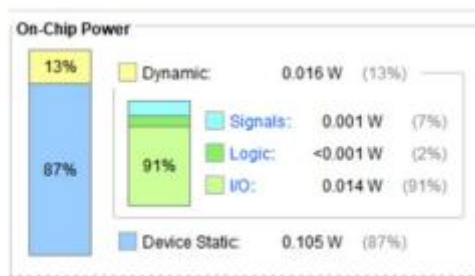
Fig 5.2 Power analysis of a 32 bit ALU based on existing design
