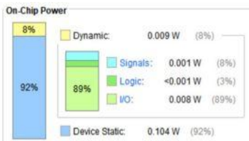
Fig 5.6 Power consumption analysis of proposed design based 32 bit ALU
