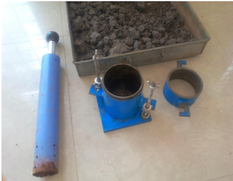
(FIG.3.3.4a) STANDARD PROCTOR TEST APPARATUS
