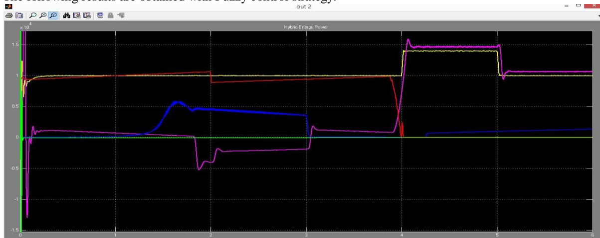
Figure16: Power Outputs of Energy Sources and Load Power with Fuzzy Controller
