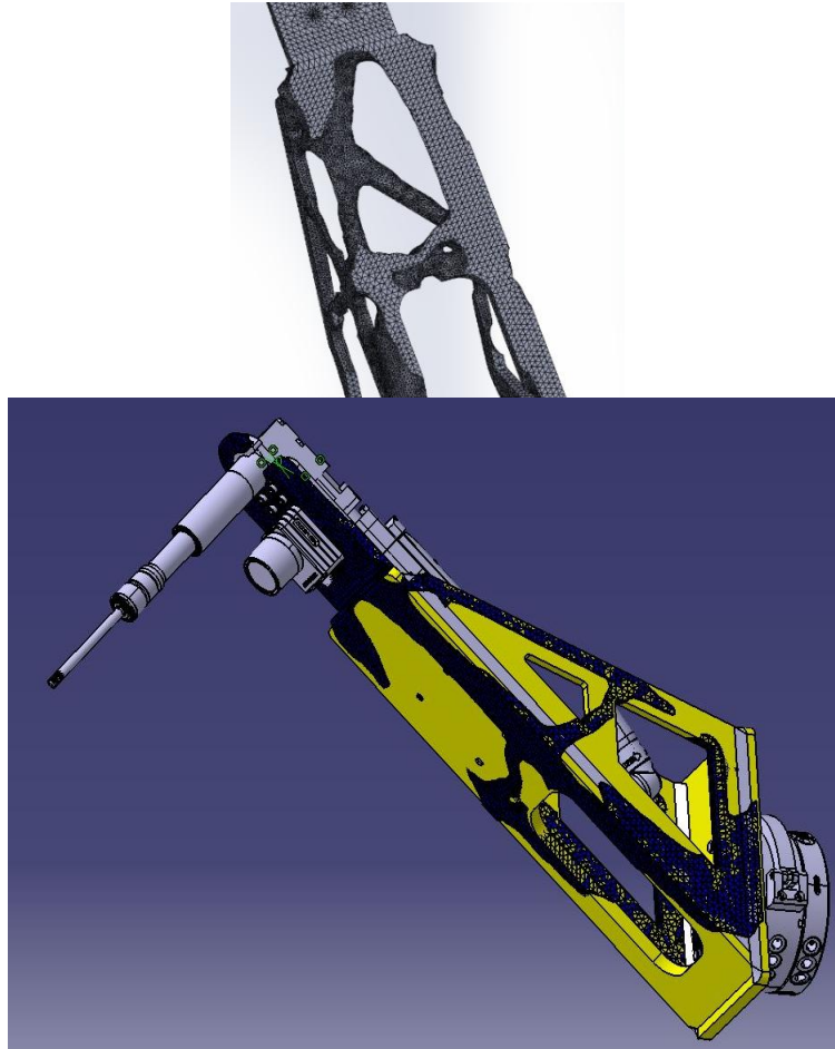
Figure12: Resulting shape after TO (left) and comparison of both shapes of gripper (right)
