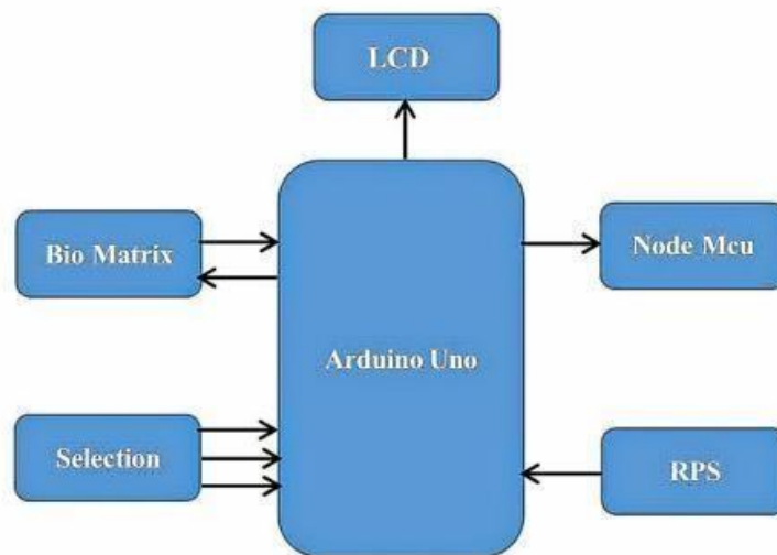
Figure 4: Block diagram of hardware working
