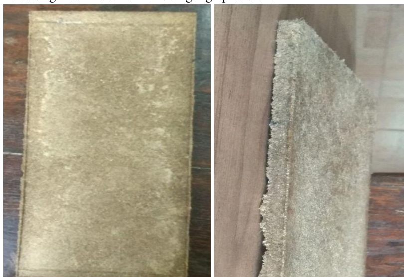
Fig 10. Hybrid Composite Panels (a)Water Hyacinth (b) Pineapple Leaves
