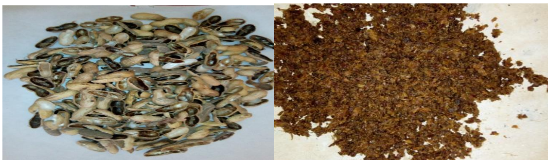
Plate I: Groundnut shell Plate II: Leached groundnut shell
