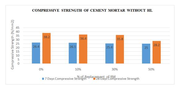
Cement cube and concrete cube specimens measuring 70.6x70.6x70.6mm and 100x100x100mm were subjected to a compression test, and six samples were evaluated to determine the average value at 7 and 28 days. According to IS 516-1959, a compressive strength test on a cube is conducted.
