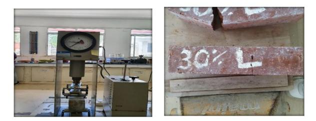
The test is carried out on concrete beam specimens of size 100x100x500mm, six number of samples were tested to get the average value at 7 and 28 days. The test is run with the IS 516-1959 code.
