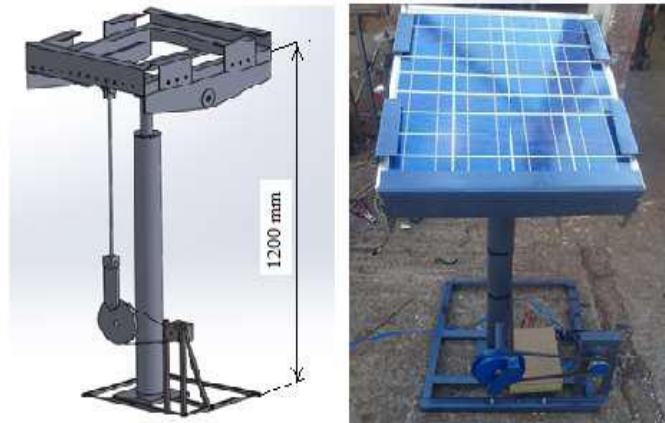
Fig- 11 (a) Model tracker; (b) Manufactured prototype
