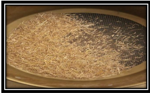
Figure 3.1 Rice Straw (600 micron) Figure 3.2 Panel Casting
