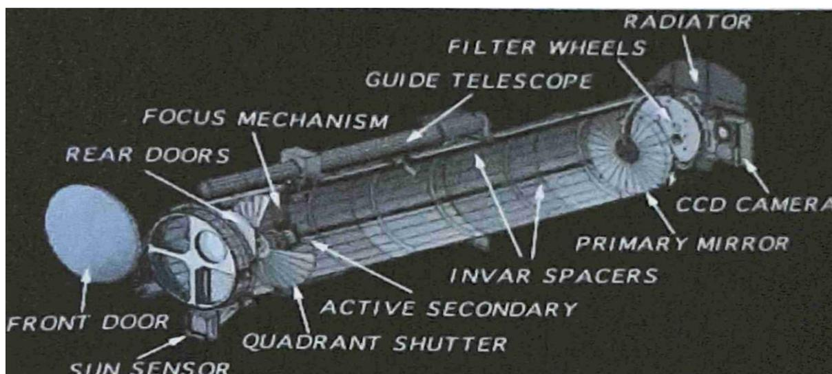
**Fig.6:** A cut-away view of the Transition Region and Coronal Explorer (TRACE) telescope is shown. The 30-cm aperture TRACE telescope uses four normal-incidence coatings for the EUV and UV on quadrants of the primary and secondary mirrors.[14]
