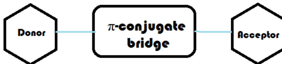
Figure 2: Structure of a typical SHG active molecule.
