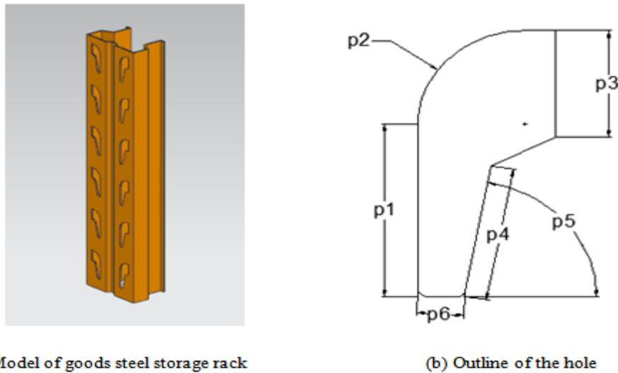
Figure 1. The model of goods steel storage rack and the outline of the hole
