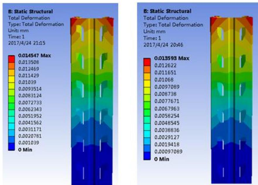
Figure 6. the total deformation of the Storage Rack Under the initial parameters (left) and optimized parameters(right)
