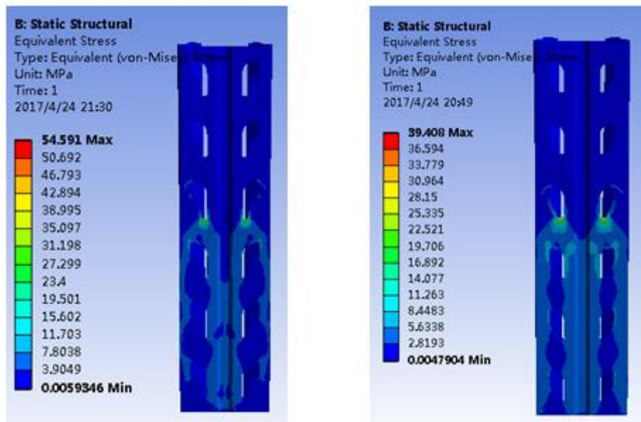
Figure 5. the equivalent stress of the Storage Rack Under the initial parameters (left) and optimized parameters(right)
