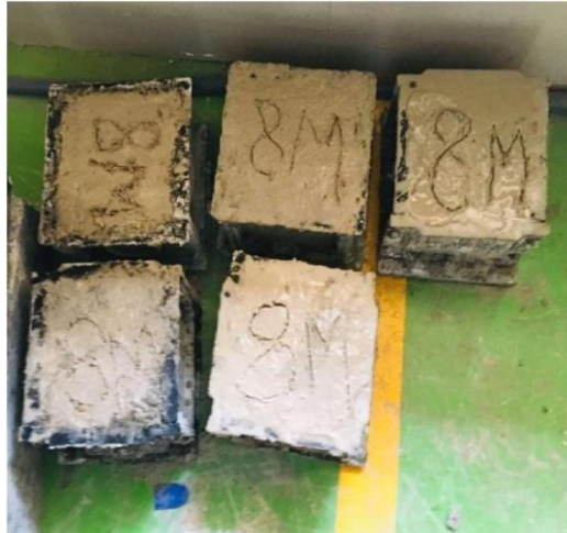
Figure 2: Cubes after Casting
