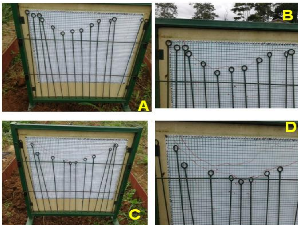
Figure 3: Estimation soil disturbance (A – D) showing on the developed profilometer
