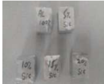
Specimen of AlSiC MMCs for density test
