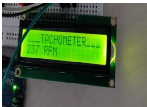
Figure 8. LCD displaying final RPM output
