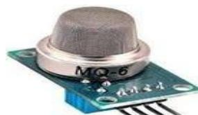
Figure 4.2: MQ6 LPG gas sensor
