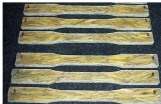
Figure 2 Tensile test specimen ASTM D638-90 standard
