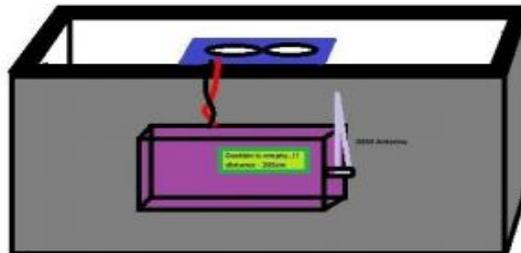
When the dustbins are about to get full, the level of garbage in the bin is detected by the ultrasonic sensors. These two sensors are set in both the dustbins to sense and send the details to the Arduino. If the bin is full, the message is sent to the municipal waste department with the location of dustbins using gsm module. The location is programmed in the Arduino code.
