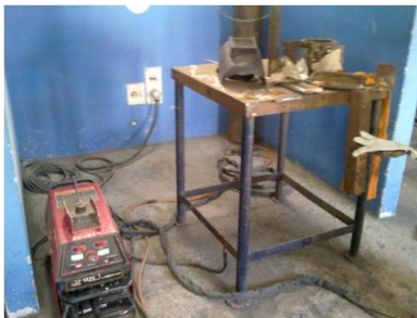
Figure 2: TIG Welding Machine Setup
