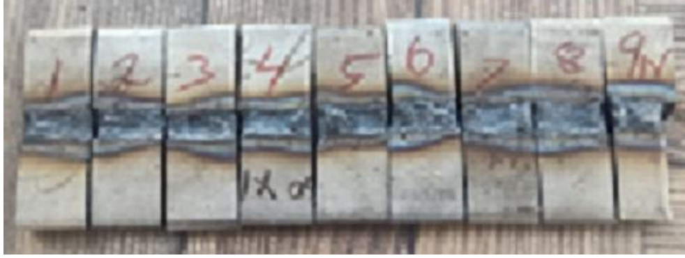
Figure 4: Hardness Test for L9 Specimens
