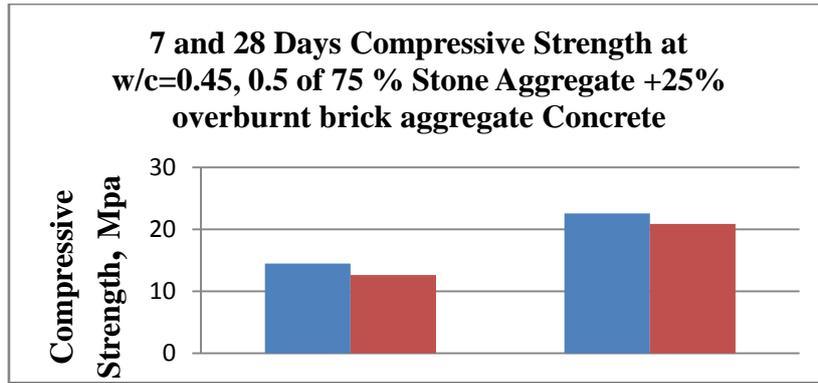
Graph 2: Compressive strength of 75% stone aggregate +25% Over-burnt brick aggregate concrete
