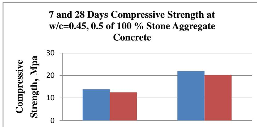
**Graph 1:** Compressive strength of 100% stone aggregate concrete
