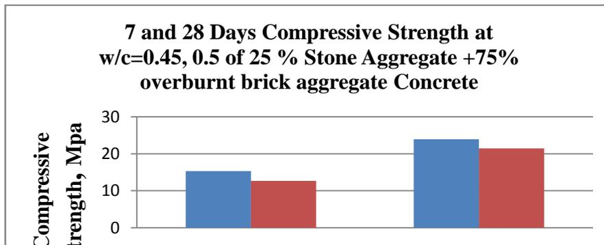
Graph 4: Compressive strength of 75% stone aggregate +25% Over-burnt brick aggregate concrete
