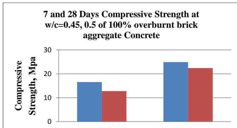
Graph 5: Compressive strength of 100% Over-burnt brick aggregate concrete
