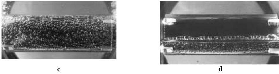
Figure 9: Modes of heat transfer in the evaporator: a) subcooled liquid heating near the entrance of the annular minichannel of LTCE evaporator; b) beginning of nucleate boiling of the saturated liquid in the annular minichannel of LTCE evaporator; c) bubble flow heat transfer; d) evaporation inside the wick, capillary suction of the liquid from the liquid rivulet at the bottom of evaporator.
