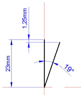
**Figure 1** Concept of switch handle thrust design
