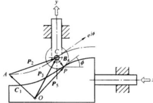
Figure 2 Design of round-end follower linear motion cam curve <sup>[4]</sup>
