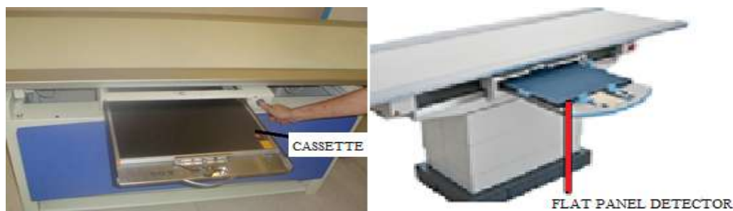
Figure 1: (a)Cassetteused in conventionalsystem, (b) Flat Panel Detector in DigitalSystems
