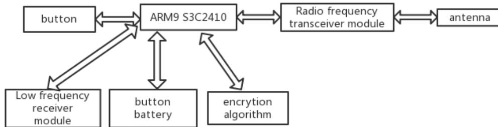
**Fig. 2 PKE“key” overall block diagram**
