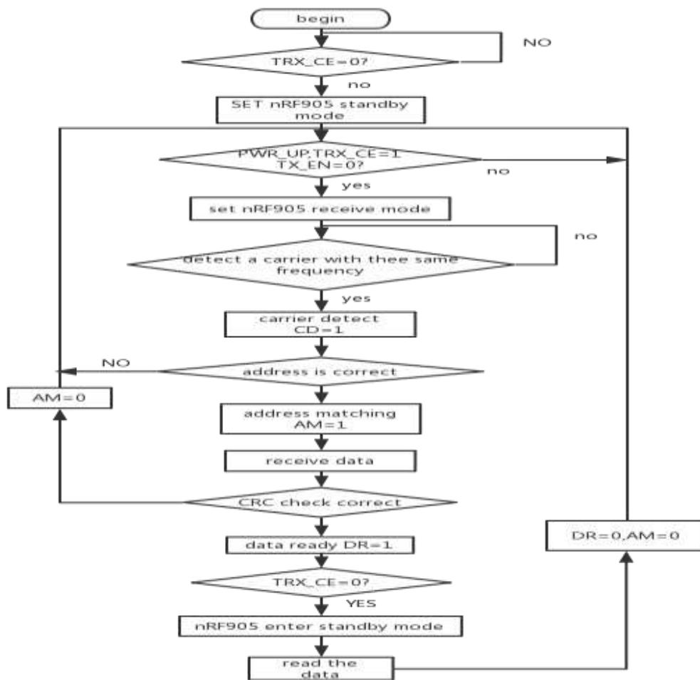
Fig. 6 Wireless receive flow chart
