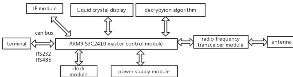
**Fig. 3 On-vehicle PKE overall block diagram**
