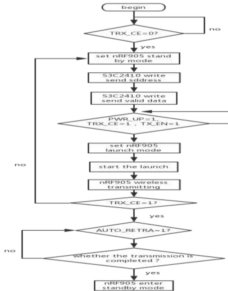
Fig. 5 Wireless transmission flow chart
