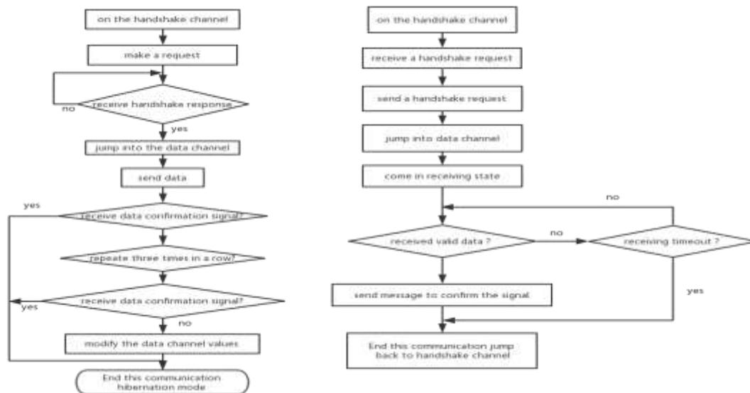
Fig. 7 Frequency hopping communication flow chart
