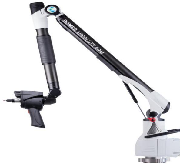
Figure 3 Articulated arm coordinate measuring machine
