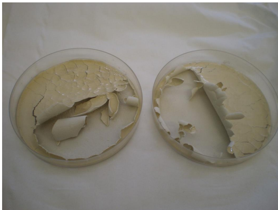
Figure 1: Picture of a PVA-MMT blend (10 mL of a 5 % w/v PVA solution and 10 mL of a 10 % w/v MMT suspension at pH = 10) after 2 days of drying.
