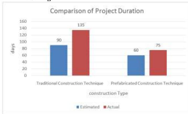
Figure 2: Project duration for both traditional and prefabricated construction technique
