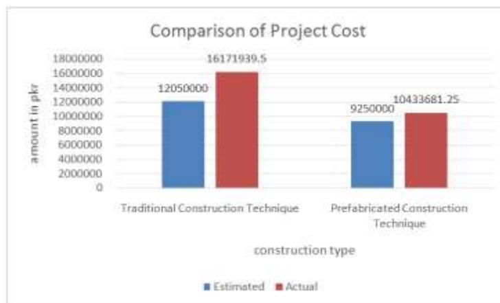
Figure 3: Project Cost for both traditional and prefabricated construction techniques
