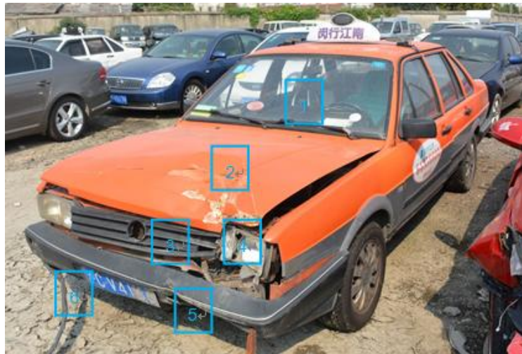
Fig. 2 The overall damage of Santana
