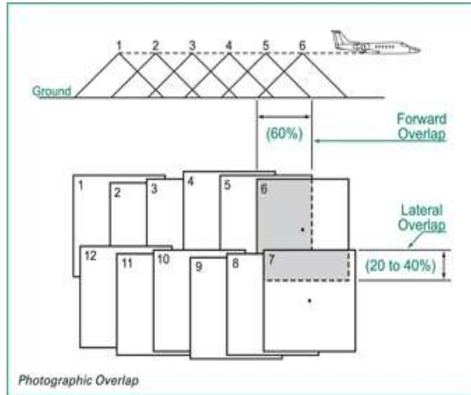
Figure 6 Example of overlapping photographs. Image obtained from <http://www.photogrammetrynews.com/2015/12/planning-of-aerial-photography-overlaps.html>
