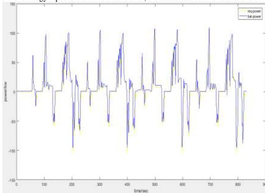
Through the calculation, the braking energy recovery rate can reach 82%, and on the basis of simple parallel control strategy, it is about 20 percentage points to prove the rationality and feasibility of the new series control strategy.
