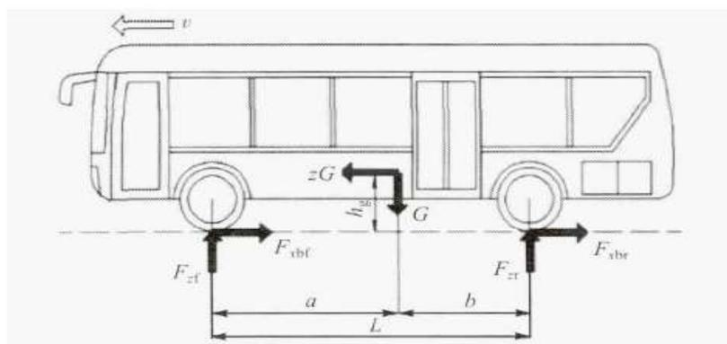
Figure 1 electric bus brake force analysis
