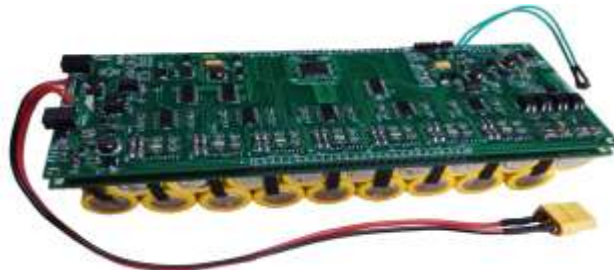
Figure 5. Balanced redundant module
