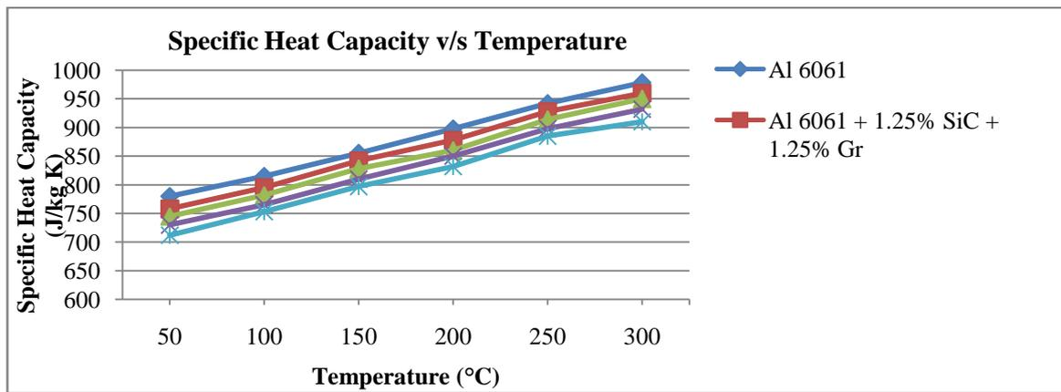
**Fig. 1. Variation of Specific Heat Capacity with Temperature of Hybrid Composites**
