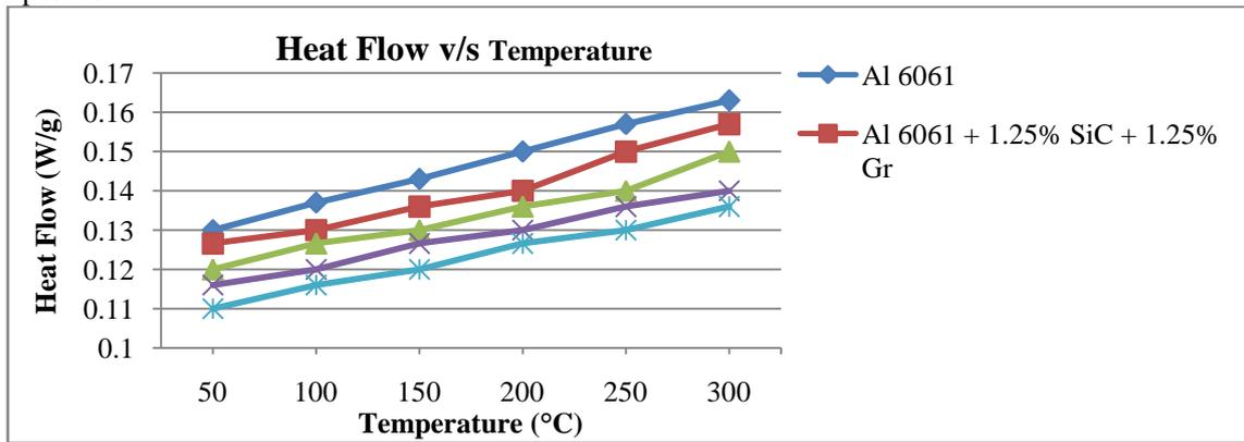
Fig. 3. Variation of Heat Flow with Temperature of Hybrid Composites
