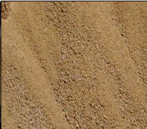
**Fig.4 :** River sand which normally used in concrete
