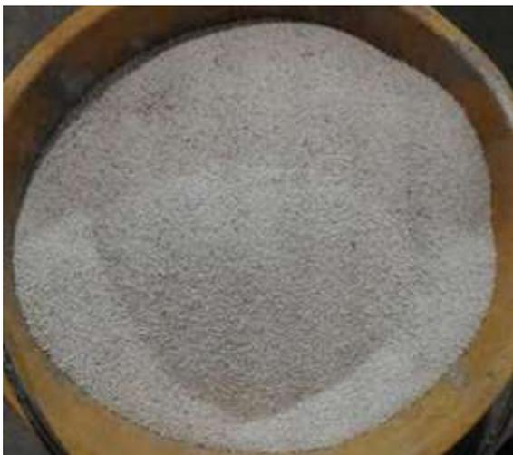
**Fig.3 :** Crushed cockle shell to be used in concrete
