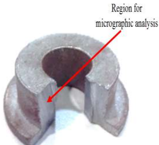
Figure 2. Residue sintered at 1200 °C in conveyor furnace.
