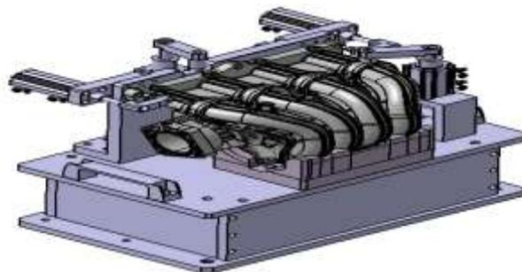
Fig 5 Intake manifold fixture
