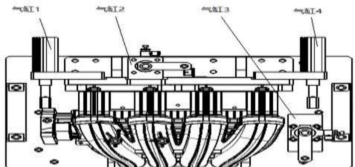
Fig 4 Cylinder in the fixture system layout
