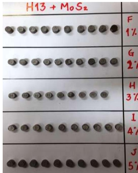
Figure 6. Sintered specimens.
