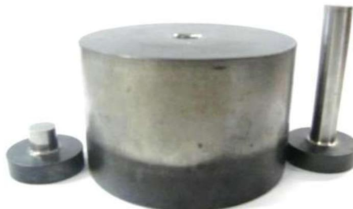
Figure 2. Compression dies for the specimens.
