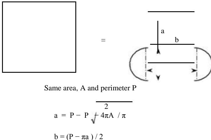
**Figure 2.1.** Geometry transformation used by Walton to reduce the three-dimensional problem to a two-dimensional problem.
