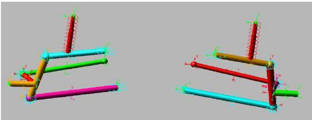
Picture 2 Wishbone type independent front suspension model
