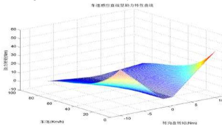
Picture 11 Three-dimension picture of linear assistance characteristic curve
