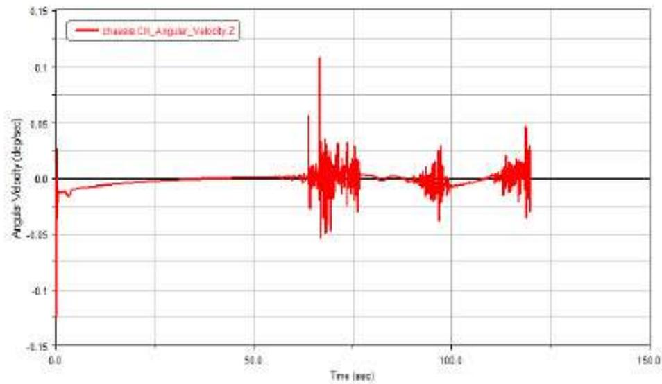
Picture 8 Curve of centroid yaw velocity
