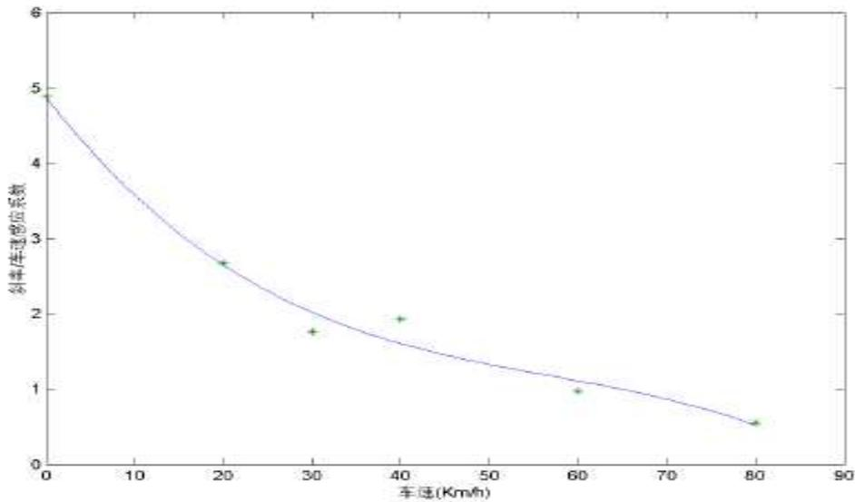
Picture 10 Relations between slope and speed
