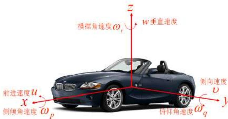
Picture 1 Three-dimensional vehicle coordinate system
